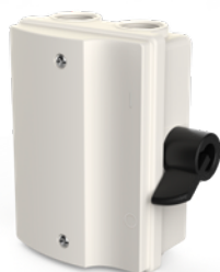
Safety Switch SSB/SSB EMC With lockable toggle. Two M25 bushings included. SSB EMC is copper-sheathed.
